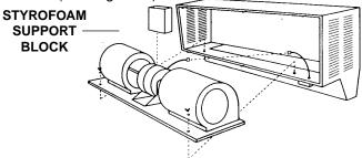
Figure 4 - Removing Motor/Blower Assembly
